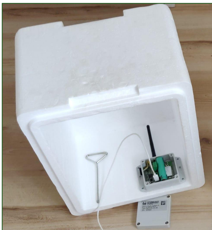
Example of delivery package with installed monitoring unit
